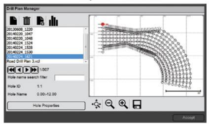
The drill plans available are listed in the middle of the left side of the dialog. The currently selected drill plan is highlighted in blue and is displayed in the map window to the right.
